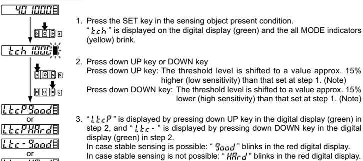
Note: The shift value of approx. 15% is an initial value. The shift value can be change to display in percent [Approx. 0~999% (unit 1%)] or incident light intensity [0~9999 (Unit 1)]. For setting the shift amount, refer to **<PRO 1: Shift amount setting>** in **[12] PRO MODE**.
