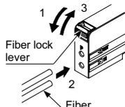
Notes: 1) In case the fiber cables are not inserted to a position where they should stop, the sensing range is reduced. Since a flexible fiber is easily bent, take care when inserting the fibers.
